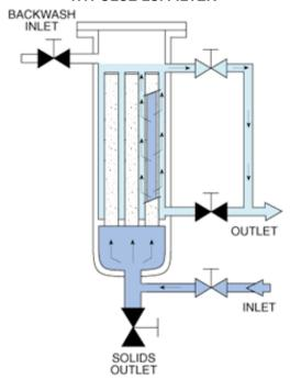
The accumulation of solids on the inside surface of the filter elements is followed by backflushing to remove the solids as highly concentrated slurry. This process is as simple as flushing slurry through a pipe.
