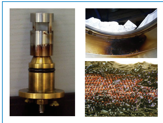
Figure 1 – Varnish on a bearing (left). Stuck valve due to varnish (top). Varnished pencil filter (bottom).
