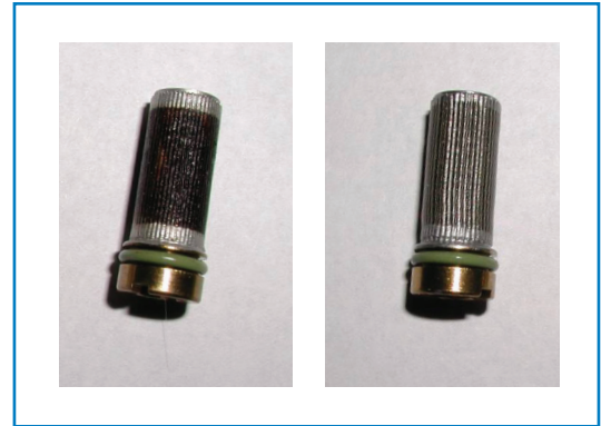
Figure 6 – Varnished servo valve before and after 45-days of electrostatic cleaning.
