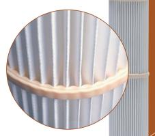
BHA iPLAS is available only with CLARCOR Industrial Air pleated filter elements. Molded polyurethane top is available in a variety of styles and sizes to fit a wide range of tubesheet holes. Other materials or designs are available for higher temperatures and unique applications.
