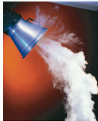
Standard hood design allows smoke bypass.
