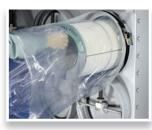
Bag-In / Bag-Out Option provides clean, safe, easy removal of fine, hazardous or difficult-to-handle dusts.
