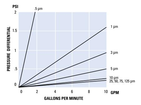
This chart represents the typical flow rate per 10" cartridge length. The test fluid is water at ambient temperature. Extrapolations for multiple lengths tend to be linear, but as flows increase the differential pressure across the housing becomes more apparent.
