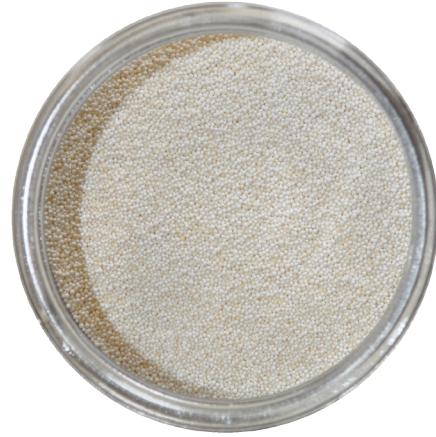
(Resin beads are clean and will not migrate or add anything to the fluid)
