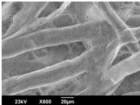
Figure 3: UAS Nanofiber Filter 600x
