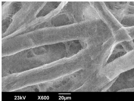
Figure 3: UAS Nanofiber Filter 600x
