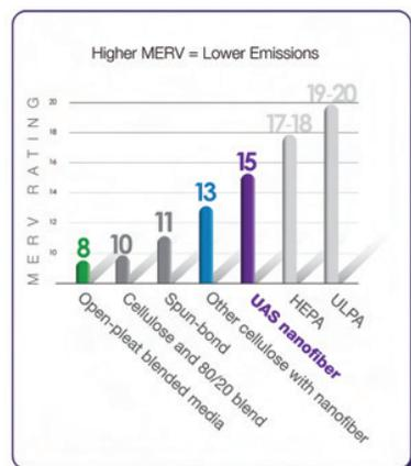
Figure 4: MERV ratings compared with filter type
