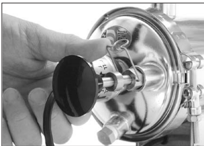
Step 1 - Lift wiper clip up
